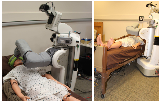
Fig. 1: Using this system, the PR2 and Autobed configured themselves for the wiping mouth task. The system raised Autobed so the PR2 base could fit underneath.
